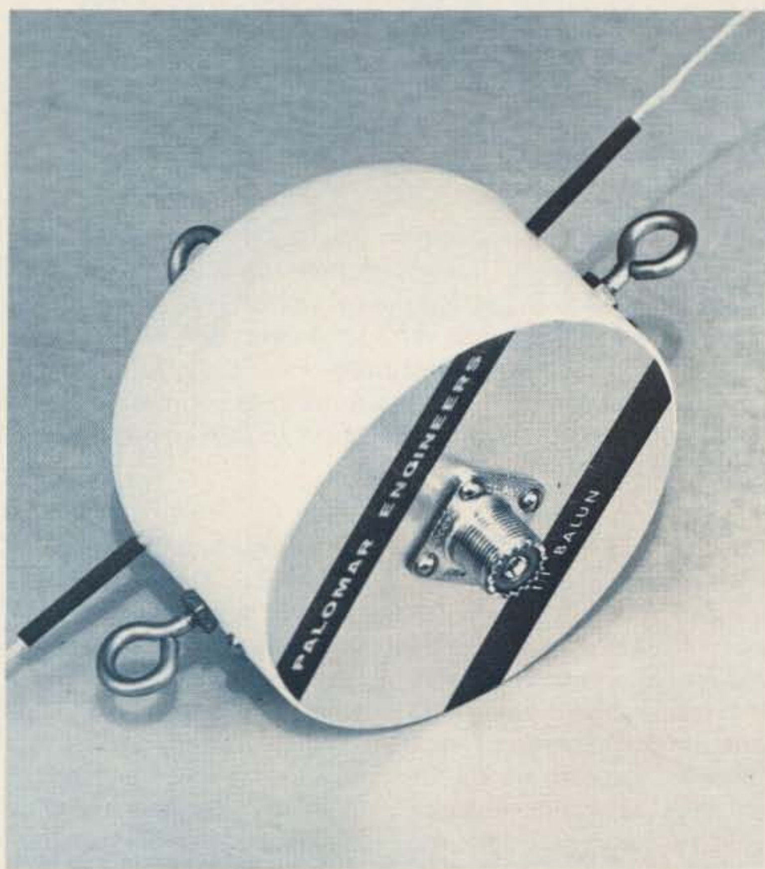
This Palomar balun is designed to match unbalanced coaxial line to balanced dipole antennas over the range of 1.7 to 30 MHz. According to the manufacturer, dipoles fed directly with coax cable are susceptible to cable radiation which can lead to TVI, BCI, rf feedback in the station, and noise pickup when receiving. The balun (balanced-to-unbalanced transformer) converts from the essential unbalanced coax to a balanced output by transformer action. Note the "hang-up" hook useful in supporting inverted-vee-type antennas. Baluns are made by numerous manufacturers, such as Unadilla Radiation, Kaufman Industries, Greene Insulator, and others. (Photo courtesy of Palomar Engineers)
